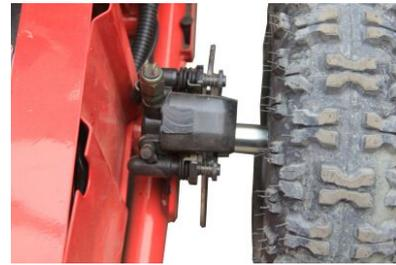
Note : Do not drive if brakes do not work properly. If you are unable to adjust and repair brakes, you may need to replace the brake friction block.
