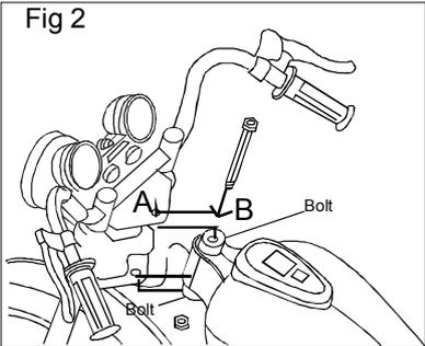
2. Connect the vehicle headlight wire to the corresponding body wire fig 3. Then align the holes in the front fork assembly with the holes in the vehicle body. Place the space rings, one on the top, one on the bottom. Then insert the hex bolt through the aligned holes, as shown in fig 2 and secure with the hex nut.
