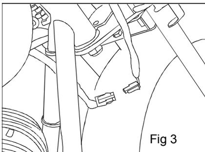
3. Locate the wires coming from the handlebar assembly and the bike and connect the terminals.
